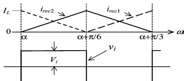
Fig. 5: Waveforms of dc output currents with AVS voltage  $V_i$ .
