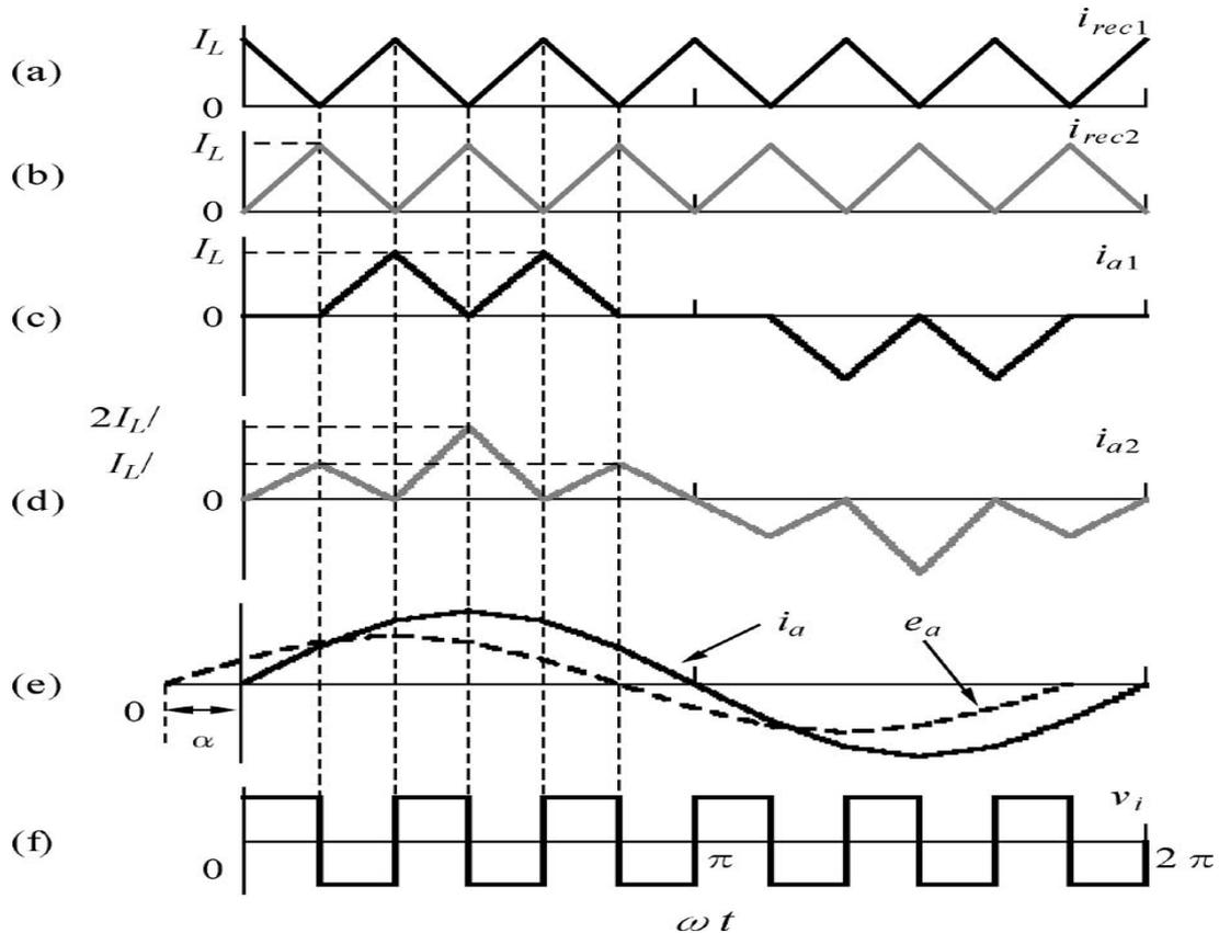
Fig. 2: Hypothetical 12-pulse rectifier current waveforms with AVS.
