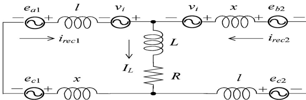
Fig. 4: Equivalent dc circuit during  $\theta = \alpha$  to  $\alpha + \pi/6$ .
