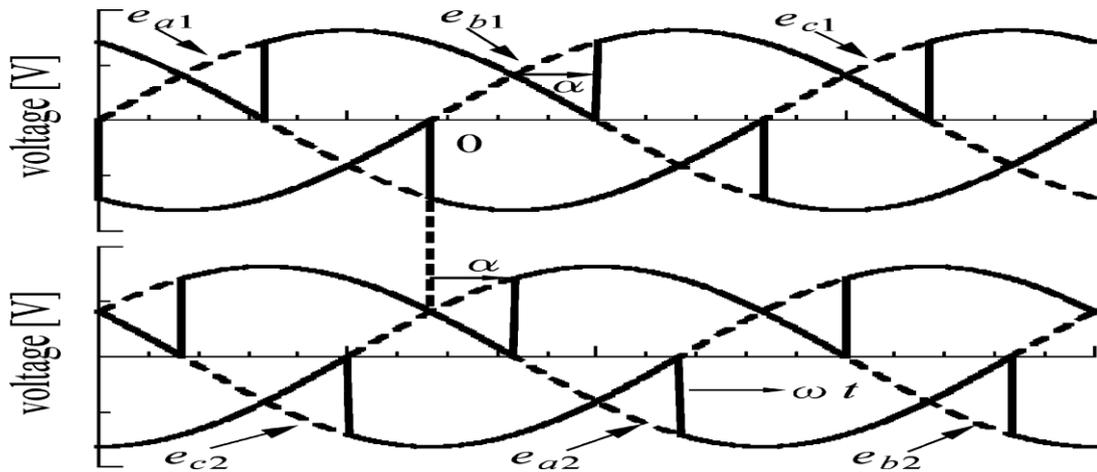
Fig. 3: Two sets of three-phase mains voltages,  $e_{a1} - e_{c1}$  for Rec1 and  $e_{a2} - e_{c2}$  for Rec2.
