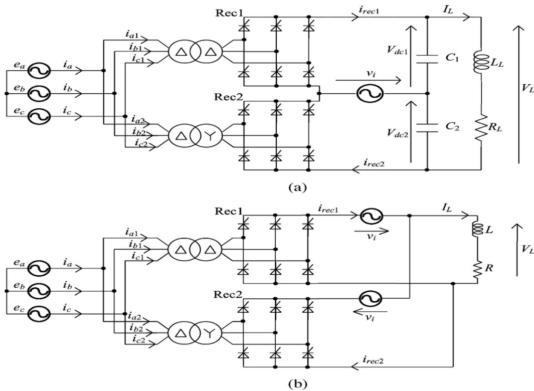
Fig.1. Configurations of phase-controlled 12-pulse thyristor rectifier with AVS  $v_i$
