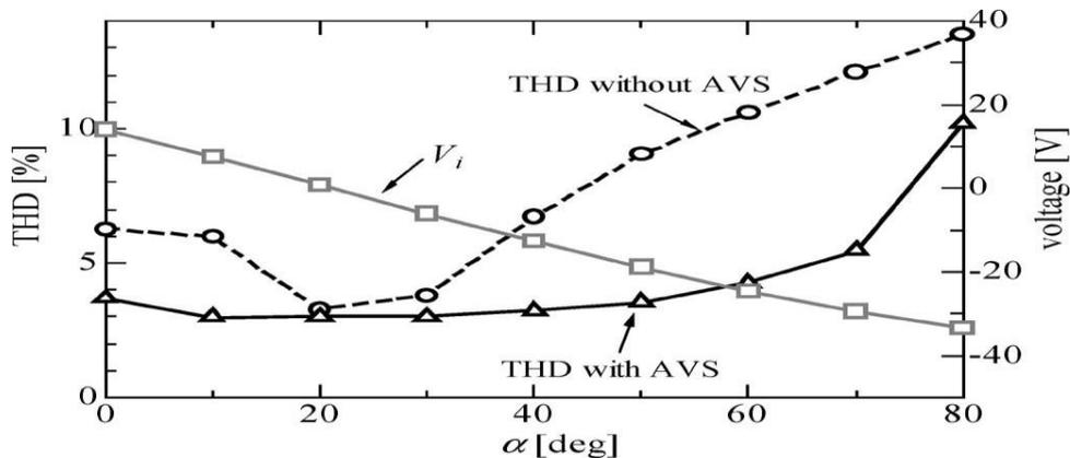
Fig. 7: Improvement in input current THD by inserting AVS with optimal amplitude.
